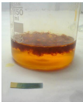
Precipitated hydrated iron(III) oxide (rust) in basic solution. Litmus paper changed its color to dark blue.
